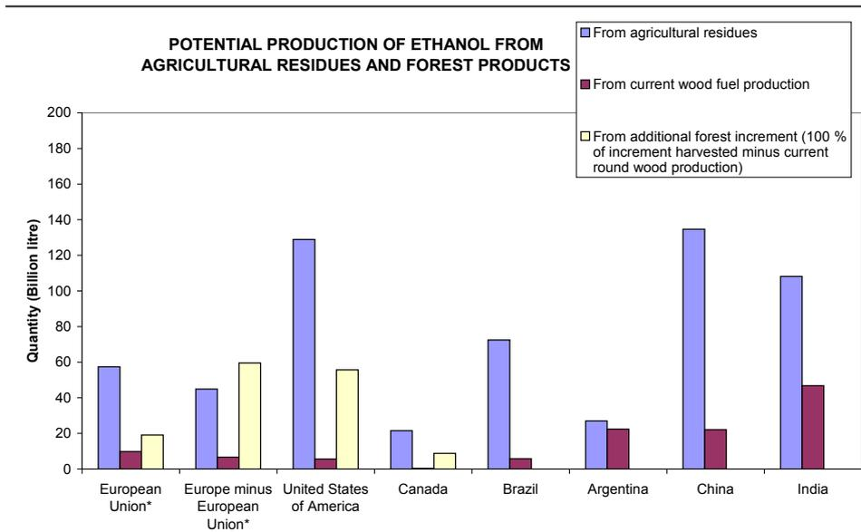
Figure 13. Ethanol production potential from agricultural residues, wood fuel production and additional wood production. Conversion technology is assumed to convert cellulose and hemicellulose. Data on forest increment is not available for Brazil, Argentina, China and India. \*European Union corresponds to EU27 minus Cyprus, Luxembourg and Malta.
