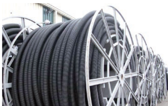
▲ Plastic pipes ready to be installed in a new district heating and cooling network.
