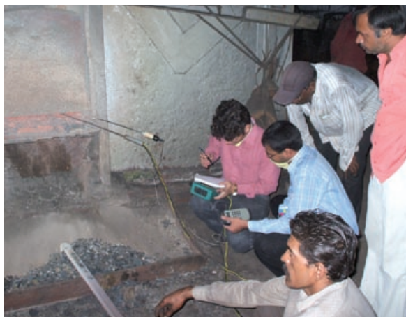
▲ Experts performing a thermal energy audit at the rolling mill cluster in Bhavnagar, Gujarat, India.
