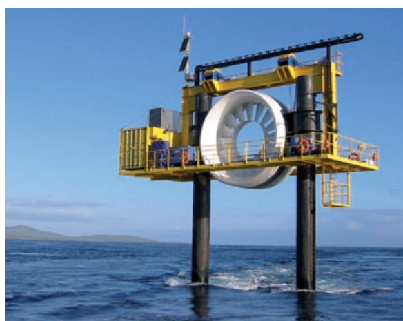
▲ An open-ring turbine prototype under test at the European Marine Energy Centre (United Kingdom).
