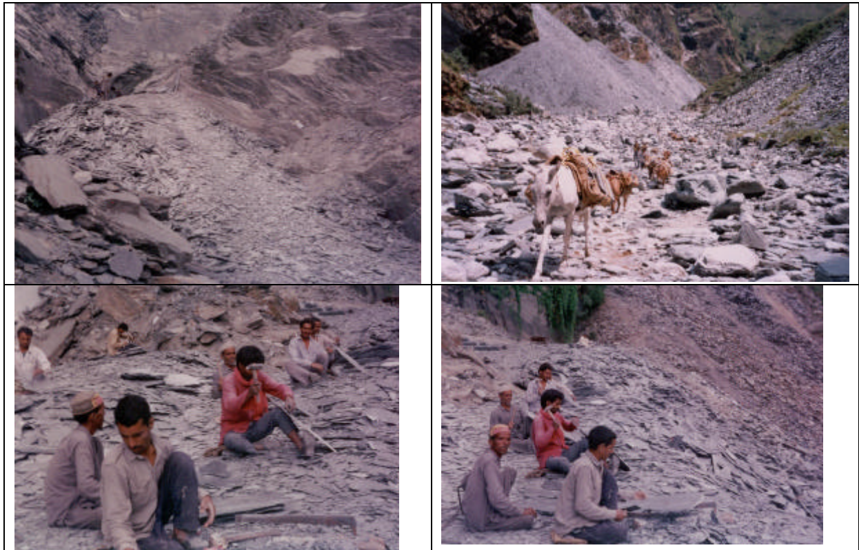
Fig.2: Manual and Age old method of Slate Mining Generates Huge Amount of Waste (Clockwise) (a) Waste Generation During Slate Extraction (b) Waste Flow into River Block Water Channel (c) Waste Generation During Slate Dressing, (d) Waste Generation During Slate Cutting
