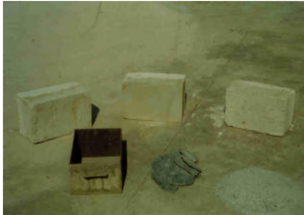
Fig.4: Concrete Blocks Made Out of Slate Waste
