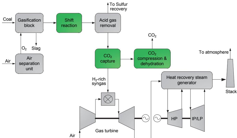
Fig.1. The block flow diagram of an IGCC power plant with CO<sub>2</sub> capture.
