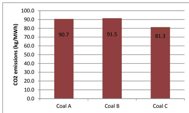
Fig.3. The specific CO<sub>2</sub> emissions from the IGCC plant with CO<sub>2</sub> capture.
