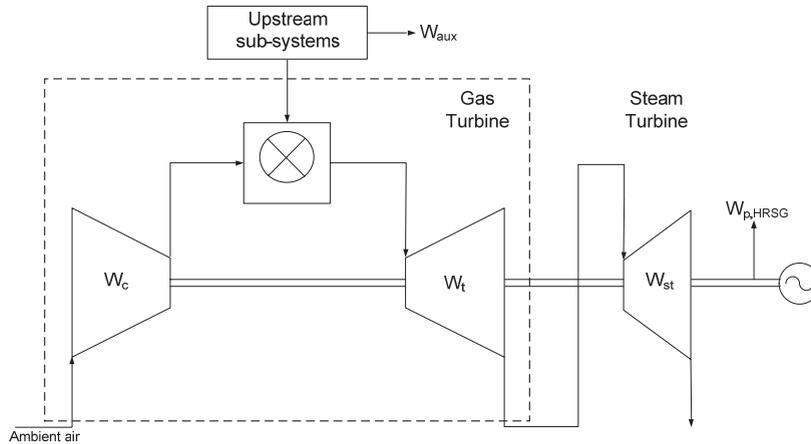
Fig.2. The boundary for efficiency calculation of the entire IGCC plant.
