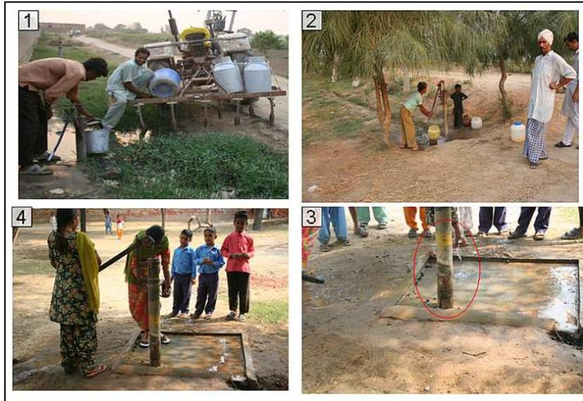
**Figure 32: Hand pumps used by people for drinking water. In image 3, notice the rusting of hand pump caused due to water quality.**
