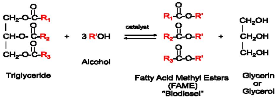
**Figure 6.** A general process for biodiesel production.
