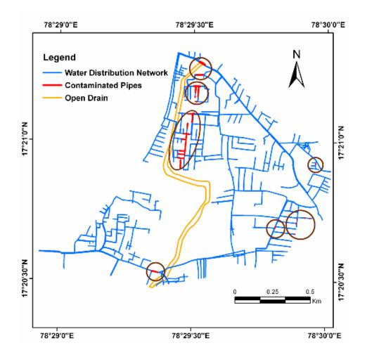
Figure 3.8 : Section of Pipes in Contaminated Zone in Water **Distribution System of Moinbagh**
