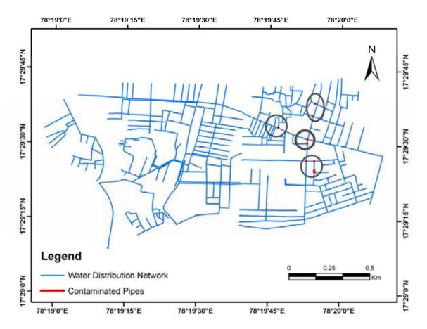
Figure 3.13: Sections Of Pipes In Contaminated Zone In Serilingampally
