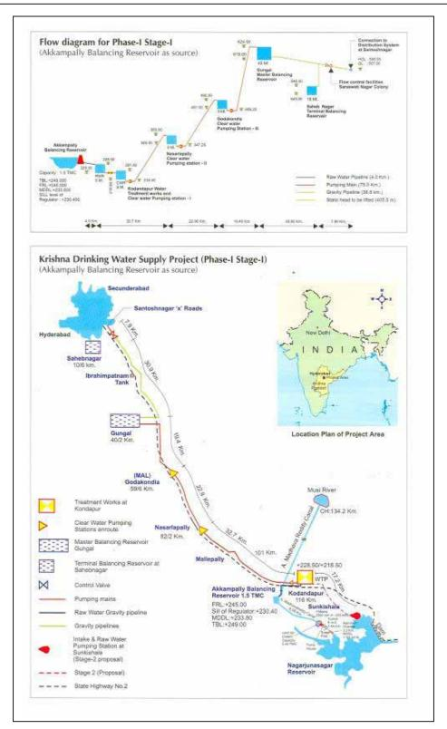
Figure 3.2: Flow diagram for Akkampally Balancing Reservoir as Source
