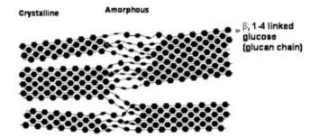
**Figure 4.** A drawing representing crystalline and amorphous regions in cellulose. The spacing between glucan chains is exaggerated to show the glucose molecules (filled hexagons)<sup>49</sup>.
