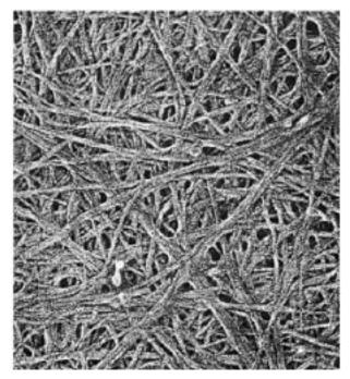
**Figure 5.** Electron microscope image of a network of cellulose microfibrils in the plant cell wall. The microfibrils are embedded in a matrix of hemicellulose and lignin which was removed by extraction<sup>25</sup>.
