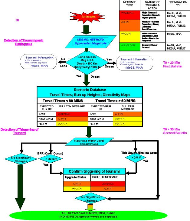
**Figure 29: Flow chart of Decision Support System and Standard Operating Procedure**
