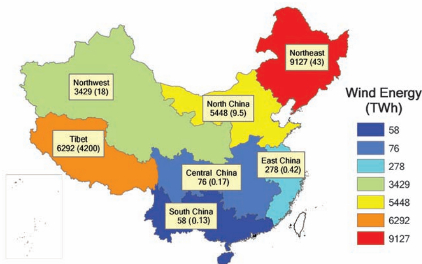
Fig. 2. Potential electricity irrespective of price that could be generated over seven electric grid areas of China mainland. The values in parentheses are the ratios of potential wind-generated electricity to current electricity production in each grid area.
