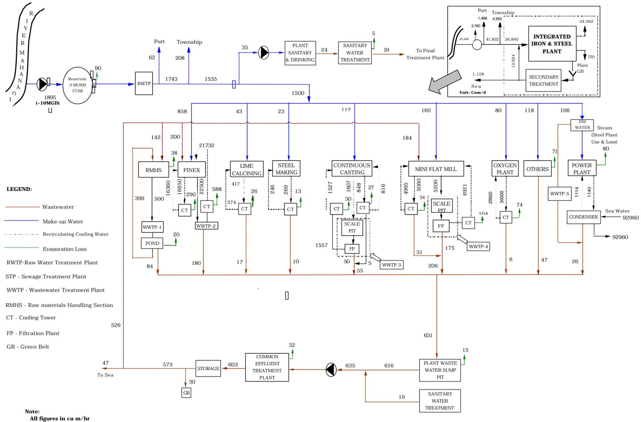
**Fig. 6-2 : Water Balance Diagram for Proposed Steel Plant at Paradip, Orissa**
