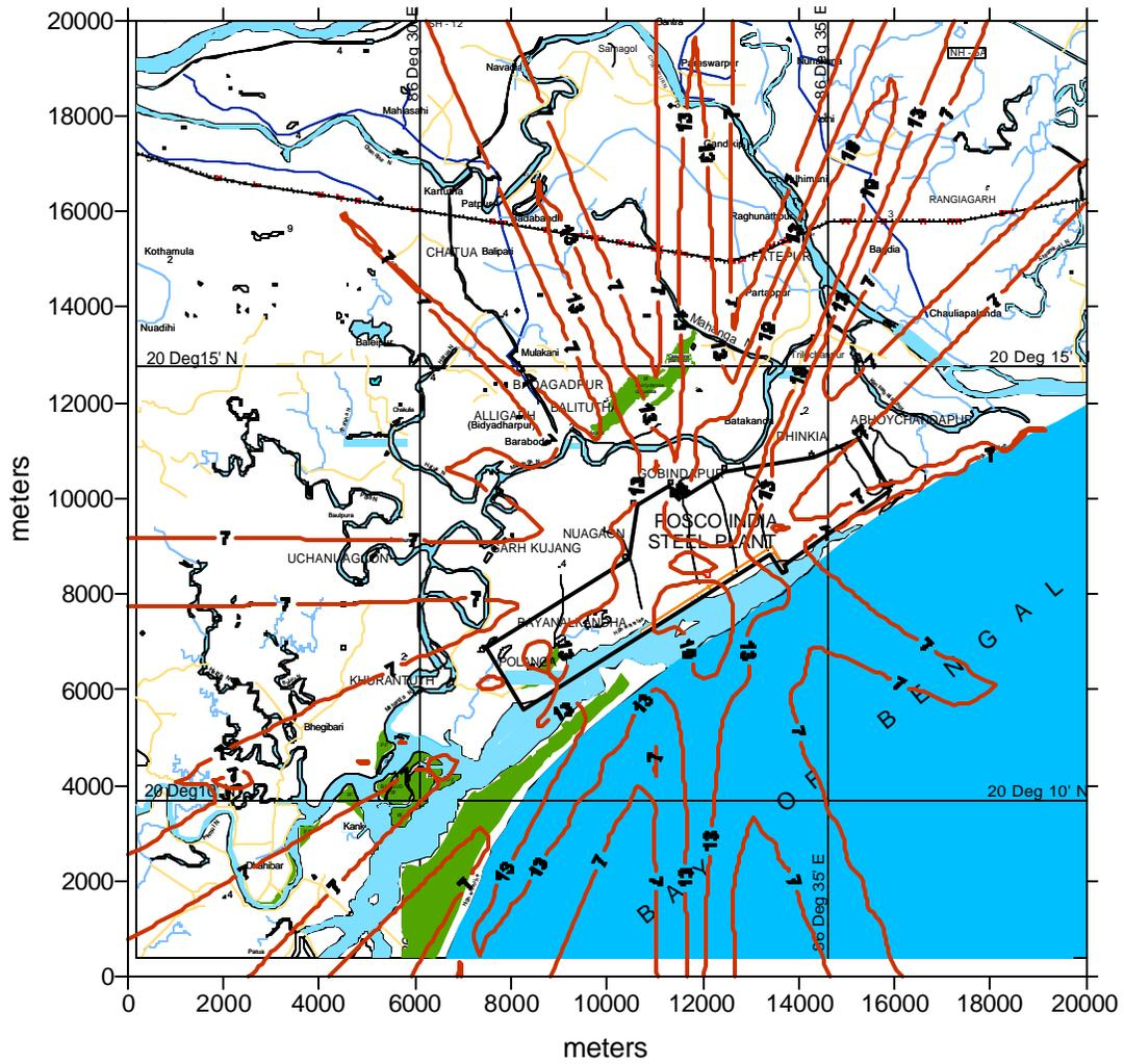
**Fig.6-9 Predicted 24 - hrly average glcs of RD in mcg/cum from the proposed 4 MTPY Steel Plant near Paradip**
