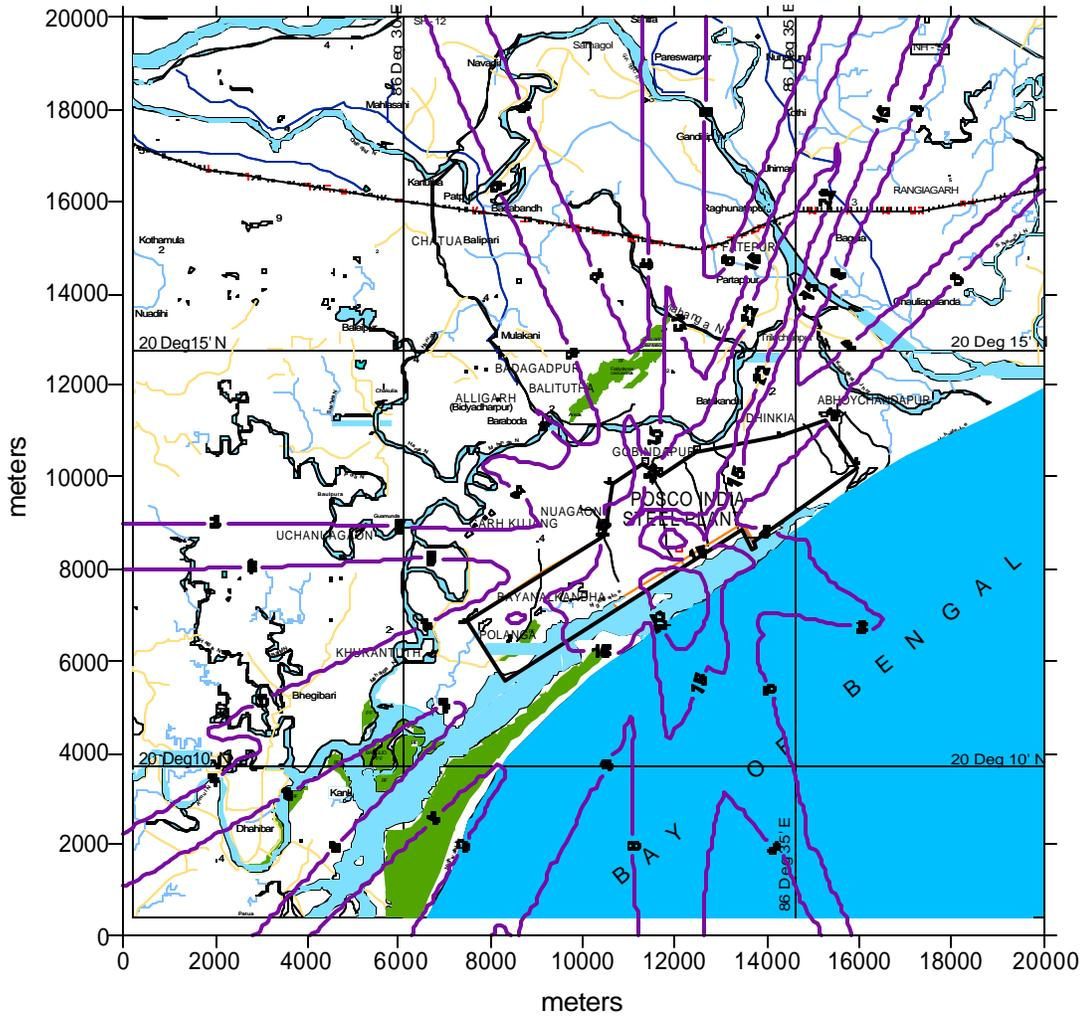
**Fig.6-11 Predicted 24 - hrly average glcs of NOx in mcg/cum from the proposed 4 MTPY Steel Plant near Paradip**
