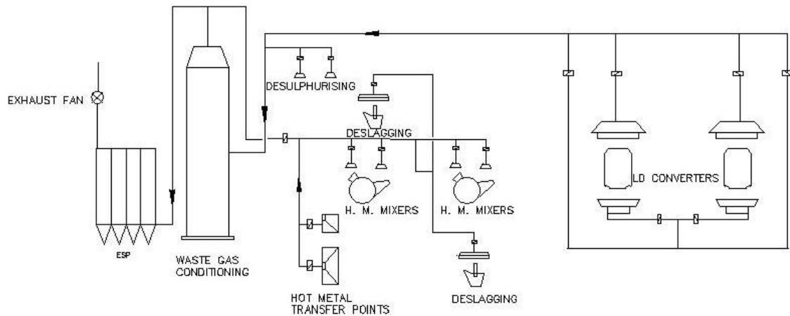
**Fig. 6-8 - A Typical Scheme of BOF Secondary Emission Control**
