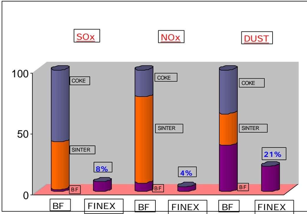
**Fig. 5-1 - Comparison of pollution level for BF and FINEX route of iron making**
