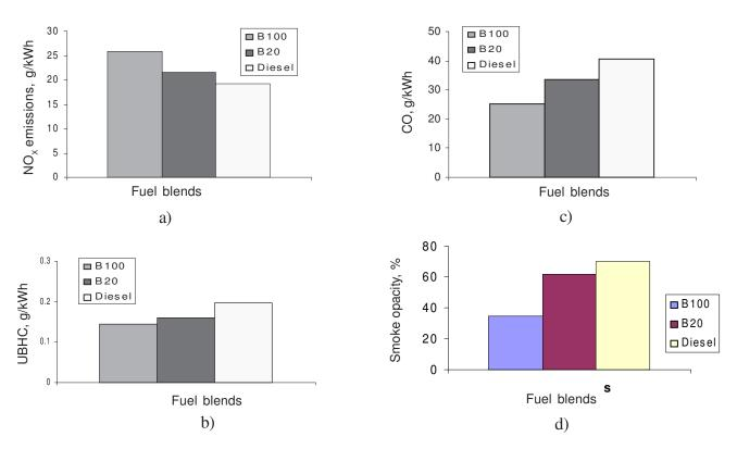
Fig. 3-Engine emissions at full load: a) NOx; b) UBHC; c) CO; d) smoke
