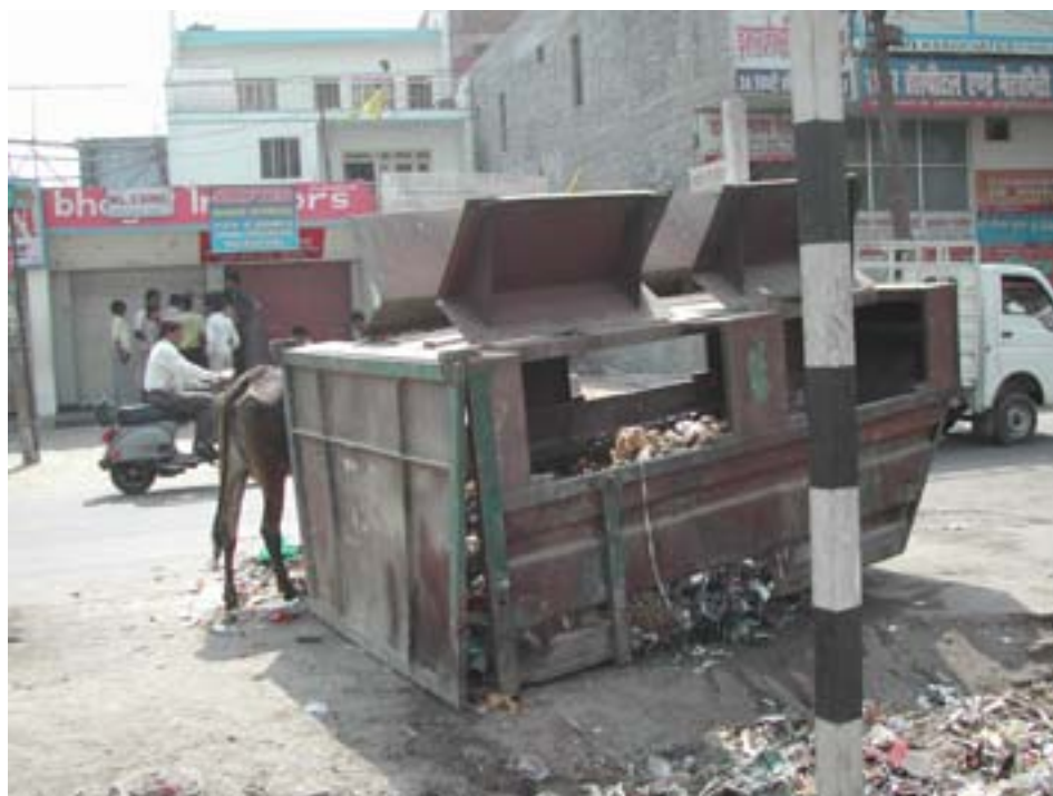
Exhibit 4.10: Dumper Placer Bin in Improper Condition
