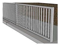
The guard railing is necessary part of the infrastructure as they segregate the pedestrian from traffic movement. The also keep the pedestrian stepping into the carriage way, even accidentally. Continuous railing not necessarily metal /MS, concrete, etc can be proposed after detailed studies such that the MS railing are not
